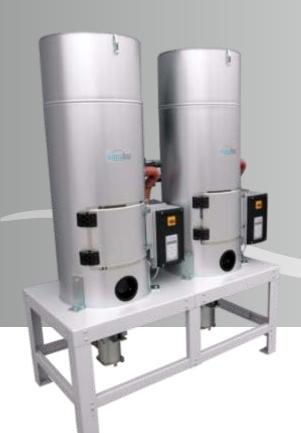
Drying hoppers are fully insulated with individual heaters and temperature setting controls. The cylindrical shape ensures uniform drying.
